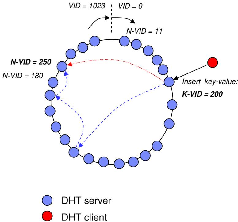
**Figure 3 - DHT example on a 10 bit VID space: the storage node of key with VID=200 is node with VID=250**
